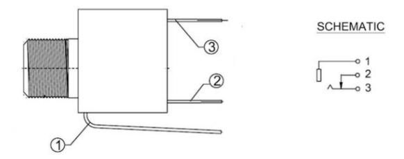
Each jack has three lugs: 1 is the ground, 3 is the signal, and 2 is a switch. When no jack is inserted, pin 2 is connected (or "normalled" to pin 3.
