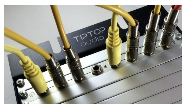
5. Testing: Begin by testing the first configuration. See the image above. In the first configuration, the red cable is feeding in a signal, and each yellow cable is distributing that signal elsewhere. This is easily tested by using an oscillator or mp3 player, and listening to the other jacks via headphones. The fifth jack is not used, as that is a switched jack. When a
