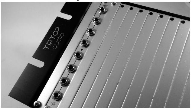
It is critically important to be able to split and distribute your modular's signals to multiple destinations, and the Al001 Multiple module does just that. Because the module takes up only 2HP, it can be placed anywhere.
