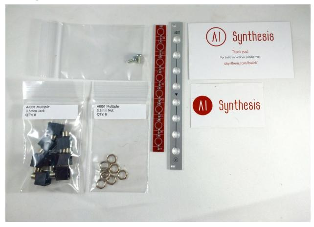
In the kit: 2 Mounting Screws, a PCB, an aluminum panel, 8 jacks, 8 nuts, a card linking to these instructions, and a sticker. Because this is a passive module, no power cable is included.
