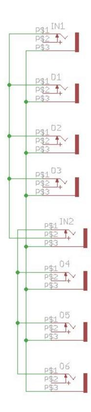
In our Multiple, only In2 uses this switched jack. When no jack is inserted into In2, signal passes from In1, O1, O2, and O3 onto O4, O5, and O6. Inserting a jack into In2 breaks this switch, and so the signal from In2 passes to O4, O5, and O6.
