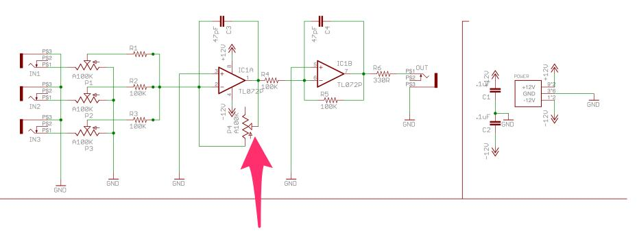
Note that on Rev 1 PCB, the third leg is connected to ground. For proper operation, the third leg of the potentiometer should be clipped (see build guide).
